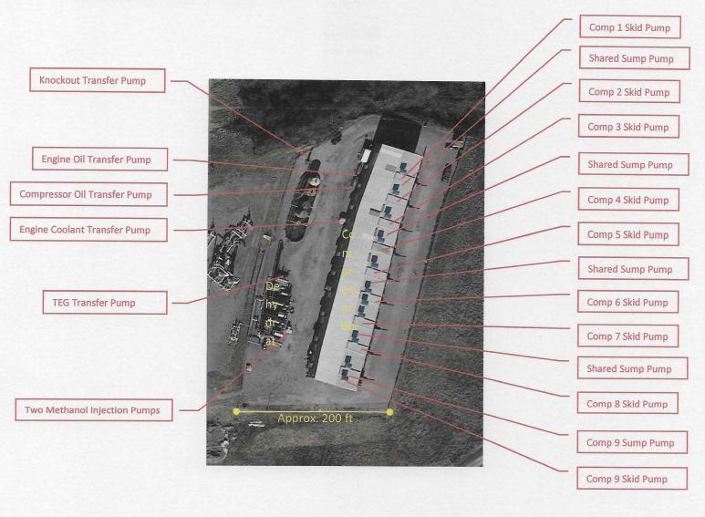
**Methanol injection pumps** – These pumps are used to inject methanol during the colder months to prevent freezing. Usage varies highly depending on the local climate. At this northern location, methanol injection is used six months per year.
